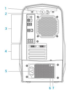
Security cable slot — Attaches a commercially available security cable to the computer.
